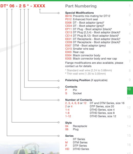
Please note that all DT Series connectors require secondary wedgelocks which are sold separately, see following pages. The wedgelocks help ensure proper contact alignment within each connector.
